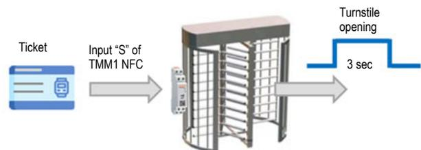
Function F- *Pulse on relay energizing with start at contact closing*
