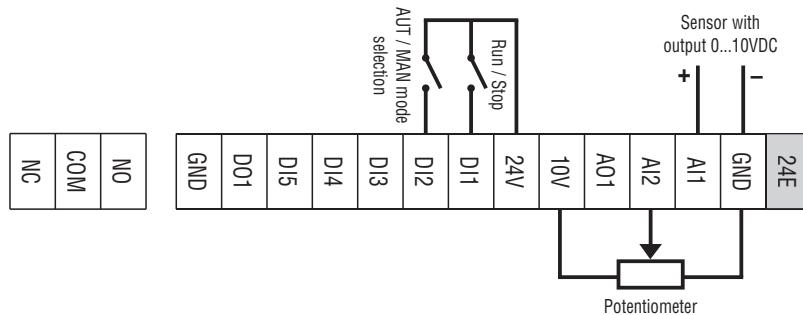
The purpose of this configuration is to manage with a digital input the switching between two operating mode:
