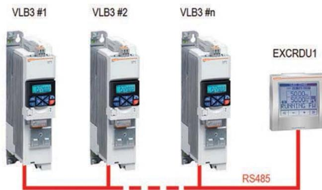
EXCRDU1 remote display unit can control up to 32 starters in contemporary at choice between variable speed drives VLB3 series and soft starters ADXL series, connected in RS485.
