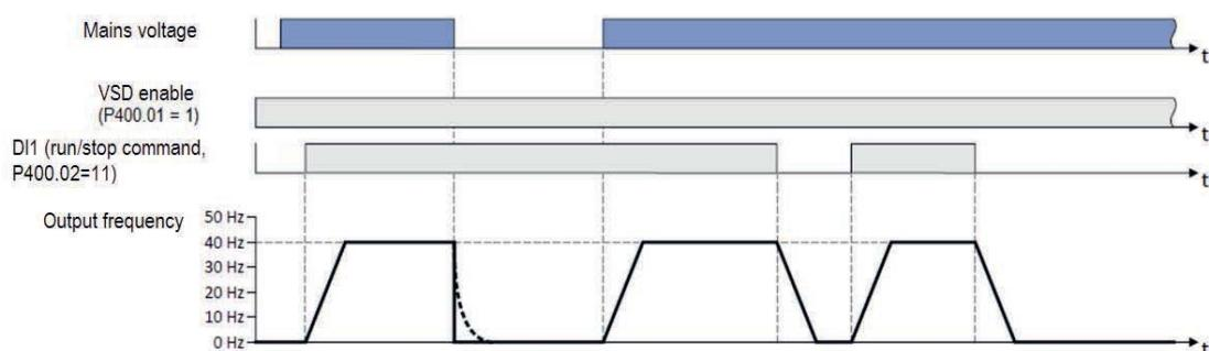
Warning! The activation of this mode causes the automatic restart of the motor at the switching on of the mains voltage of VLB3 variable speed drive. Verify that all the safety requirements are met.
