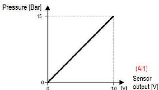
This means that: if the output of the sensor is 0V it means a pressure of 0 Bar, if the output of the sensor is 10V it means a pressure of 15 Bar, if the output of the sensor is 5V it means a pressure of 7.5 Bar, and so on.
