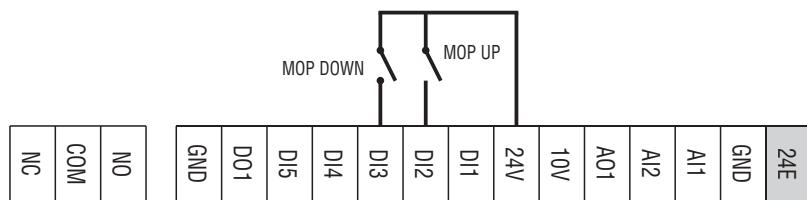
If the motor potentiometer is active as setpoint source, the frequency setpoint can be changed via the triggers assigned to two input contacts configured with the functions "MOP UP" (increase frequency) and "MOP DOWN" (decrease frequency).
