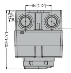
PG13.5 / M20 PG16 / M25 knockouts on top and bottom **GAZ032**
