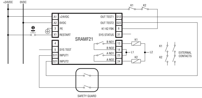
● Not necessary if set in automatic operation mode (2A)
