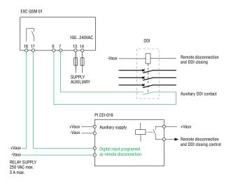
The connections coloured in GREEN, in addition to the GSM Modem, represent the only wiring necessary for the adaptation.
