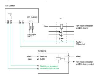
EXC GSM 01 $\operatorname{modem}$  wiring diagram with other interface protections (PI) with remote disconnection input to be supplied.
