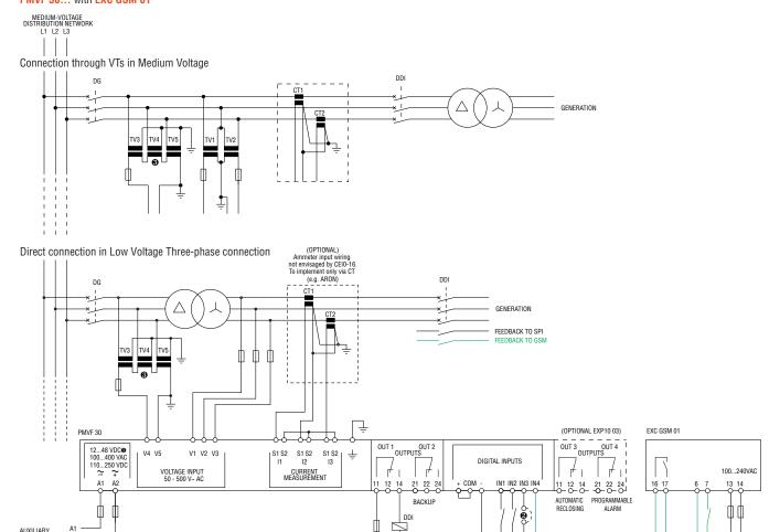
① Only for PMVF 30 D048. ② Local control choice.. ③ VT in MV for residual voltage measurements.
