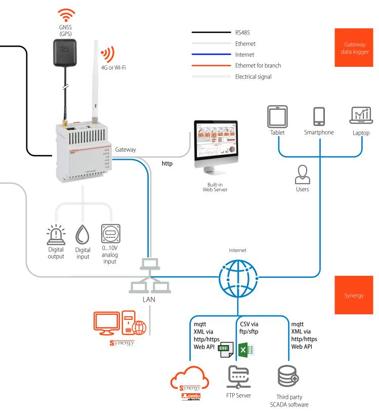
**Synergy** by LOVATO Electric is an energy monitoring and analysis system with a professional, flexible and integrated approach from an Industry 5.0 perspective. Thanks to the LOVATO Electric **measurement devices** equipped with a communication port and through the web-based supervision platform, it is possible to monitor real time measurements, consult graphics, receive alarms, export customized reports and carry out commands and settings.
