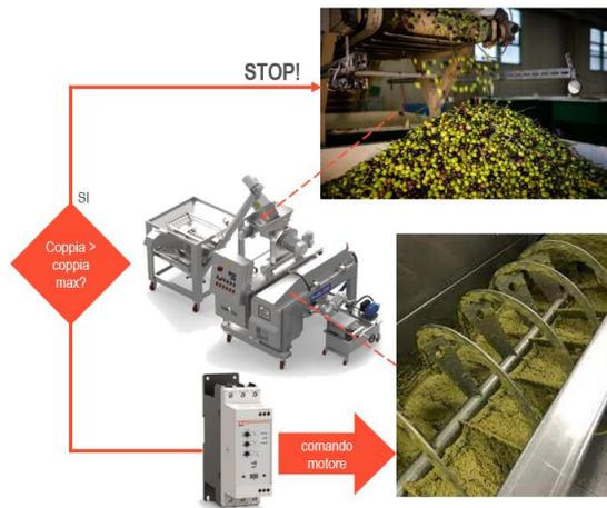
It is used to signal that the mechanical load is at a guard level and it is not possible to further increase the load.
