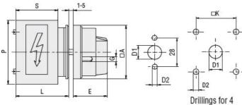
Drillings for 4 screws fixing (4V version).
