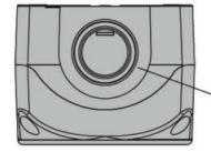
Knockout for M20/M25/PG13.5/PG16 (on top and bottom)
