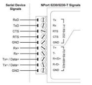
**NOTE** The NPort 5232/52321/5232-T/52321-T have 2 RS-422/485 ports. The pin assignments are the same as the NPort 5230/5230-T's port 2. Refer to the "NPort 5200 Series User's Manual" for more details.
