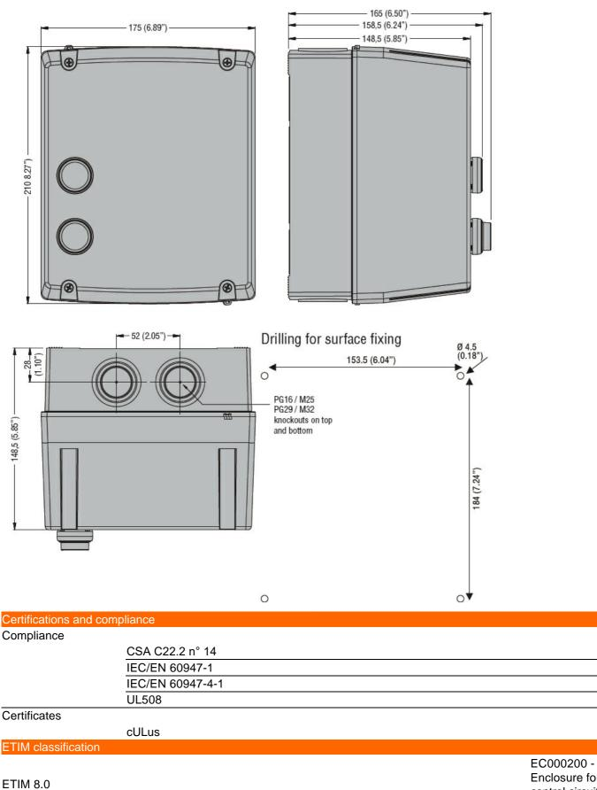
Enclosure for control circuit devices
