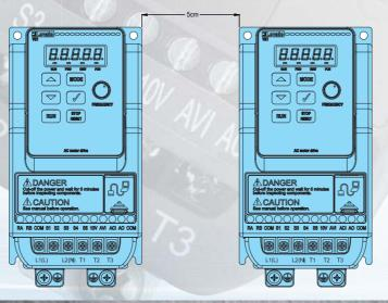
When more than one motor drive is installed side by side in a control panel, provide sufficient air circulation space of at least 5cm in order to ensure proper cooling effect.
