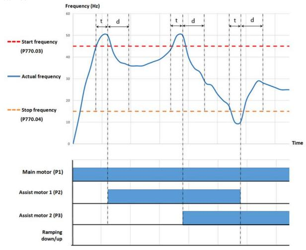
d = settling time P770.05t = start delay P770.06
