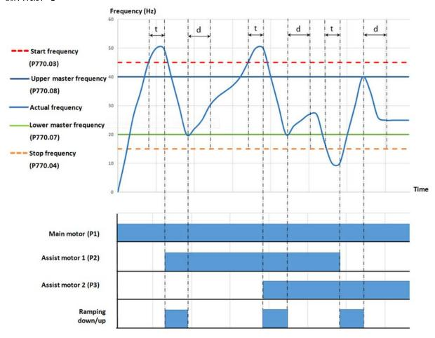
d = settling time P770.05t = start delay P770.06
