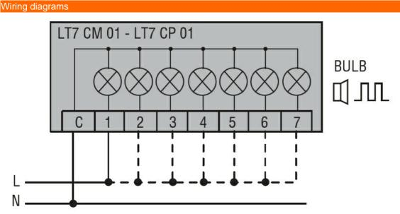
Connect terminals C and 1 as indicated to power the first module. If other modules are fitted, the respective terminals must be connected accordingly.
