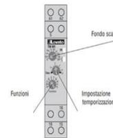
In this example the first trimmer is set to 1s and the second trimmer is set to 5, this means that 50% of the end scale must be counted, that is 0.5s.
