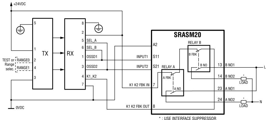
Example of connection of the SRASM20 relay with safety light curtain in MANUAL operation mode.
